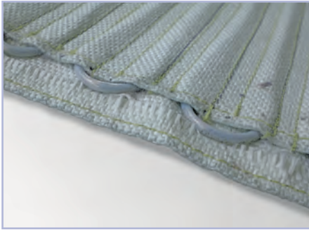
Figure 8: Fibre glass tissue with PTFE heating conductor
