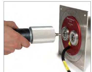
4. Heated lines are connected and secured with the coupling nut
