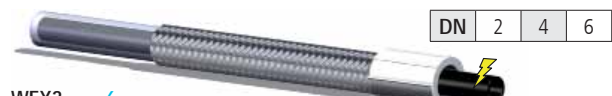
WEX3 ___ 6 PTFE basic hose with sleeves and exchangeable PTFE hose (protruding 500 mm on both sides)
