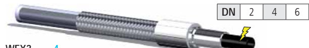
WEX3 ___ 4 PTFE basic hose with stainless steel tube ends 1.4571 and exchangeable PTFE hose (protruding 500 mm on both sides)
